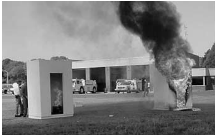
In this demonstration, two identical structures were subjected to identical fires. The structure on the left, coated with an intumescent paint, survived.
